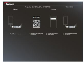
b) Connect the projector and your smart device with a USB cable. Your smart device's screen will be automatically mirrored to the projector.
