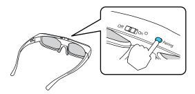
The status light on the glasses flashes green and red. If pairing is successful, the light turns green for 10 seconds and then turns off.
