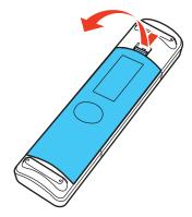
2. Insert the batteries with the + and – ends facing as shown.
