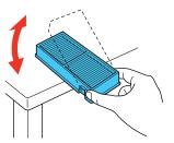
**Caution:** Do not use excessive force when tapping the air filter, or it may crack and become unusable. Do not rinse the air filter in water, or use any detergent or solvent to clean it. Do not use canned air; the gases may leave a residue, or push dust and debris into the projector's optics or other sensitive areas.
