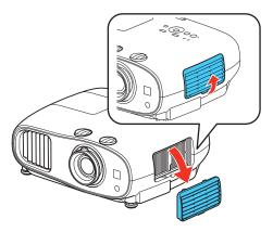
3. Pull the air filter out of the projector.
