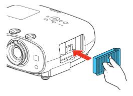
7. Attach the air filter cover as shown, and press it gently until it clicks into place.
