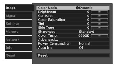
2. Press the up or down arrow button to move through the menus listed on the left. The settings for each menu are displayed on the right.
