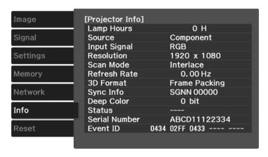
**Note:** The lamp usage timer does not register any hours until you have used the lamp for at least 10 hours. Available settings depend on the current input source.
