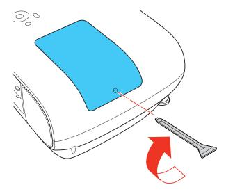
**Note:** Be sure the lamp cover is securely installed or the lamp will not come on.
