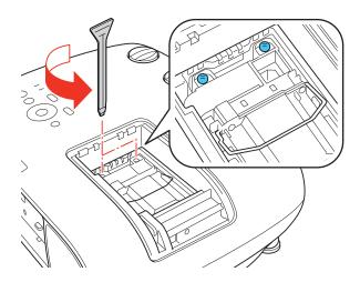
6. Lift up the lamp handle and gently pull the lamp out of the projector.
