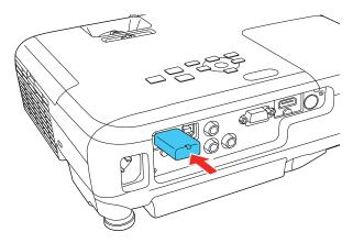
3. Attach the wireless LAN module cover and secure it using the screw you removed.
