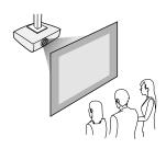
Wherever you set up the projector, make sure to position it squarely in front of the center of the screen, not at an angle, if possible.
