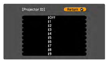
4. Press the arrow buttons on the remote control to select the identification number you want to use for the projector. Then press **Enter**.
