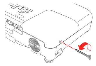
**Warning:** If the lamp is broken, glass fragments may be loose inside the lamp chamber. Be careful removing any broken glass to avoid injury. If the projector is installed on the ceiling, stand to the side of the lamp cover and not underneath it; pieces of glass could fall into your eyes or mouth when you open the lamp cover.
