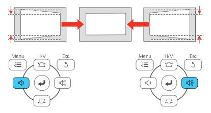
Note: The horizontal keystone adjustment buttons are labeled Wide and Tele on the VS250.
