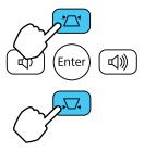
3. Press a keystone button on the projector's control panel to adjust the image shape.
