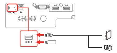
**Note:** Do not connect a USB hub or a USB cable longer than 10 feet (3 m), or the device may not operate correctly.
