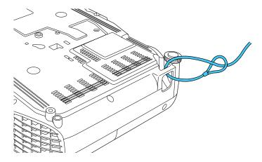
**Note:** Do not pass drop-prevention cables through the security cable attachment point when mounting the projector on a wall or ceiling.
