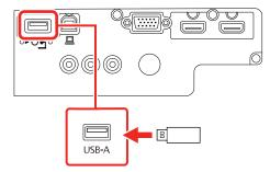
**Note:** Connect the flash drive directly to the projector. Do not use a hub or your settings may not be saved correctly.
