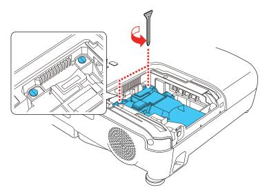
6. Grasp the raised section of the lamp and gently pull the lamp out of the projector.
