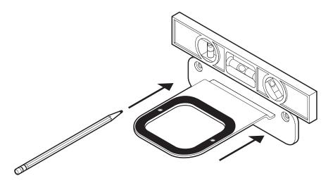
2. If using wall anchors, use a 5/16" drill bit to drill 2 pilot holes and then insert the wall anchors. Refer to the wall mounting information below for guidelines. Otherwise skip this step.
