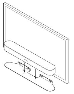
8. Insert and tighten Beam to the bracket using the mounting screws.
