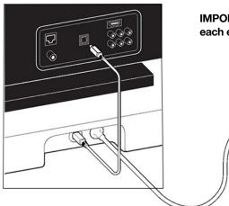
IMPORTANT: Remove the protective caps from each end of the optical audio cable.
