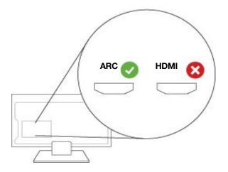
2. Connect the HDMI cable to the TV's HDMI ARC port.
