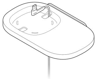
6. Press the bottom cover firmly onto the shelf until it snaps into place, carefully aligning the pins. Plug the power cord into the speaker and place the speaker on top of the shelf.
