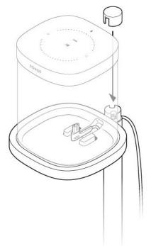
6. Press the power cord into the stem, working from top to bottom. Pull the excess cable down from the base.
