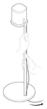
7. Tilt the stand forward slightly to wrap the excess cord around the bottom of the base. Plug the speaker's power cable into the wall and enjoy the music!
