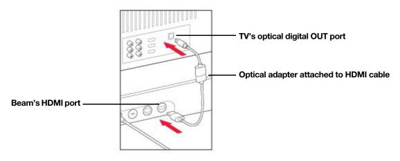
**Note:** The optical adapter's port is "D-shaped"—make sure the connector aligns correctly into the port. Inserting the adapter incorrectly may damage the cable.
