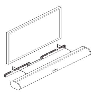
7. Slide the soundbar down so the knobs fit into the slots on the wall bracket. Make sure the touch controls are facing up, and the soundbar is fully seated.
