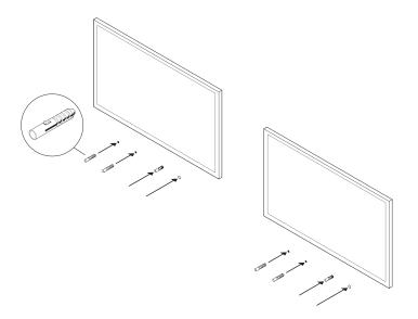
5. Place the bracket on the wall and loosely tighten the wall screws to secure the bracket. Check with a level and then tighten the screws.
