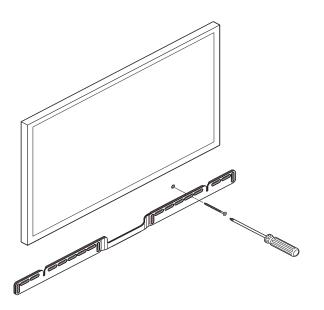
4. Position the wall mount bracket over the marked screw locations, using a level to confirm accuracy. Use a Phillips-head screwdriver or a power drill to screw the bracket to the wall, making sure the arrows in the center are pointing up.
