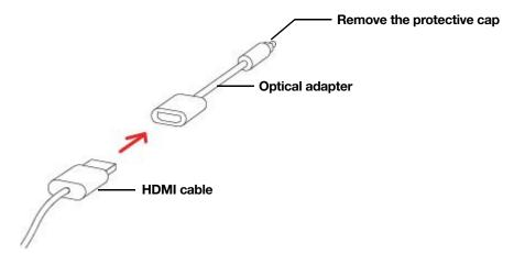
3. Connect the optical adapter to the TV's optical digital OUT port.
