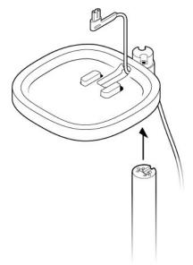
4. Use the 2 silver screws to attach the speaker platform to the top of the stem, threading the power cable carefully. Snap the bottom plate on with the power cable channel in the back, and mount the platform on the stem.
