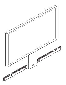
1. If your TV is wall-mounted, place the positioning guide against the wall, aligning the top edge with the bottom of your TV. There should be 5.5" (140 mm) between the top of the wall mount bracket and the TV.
