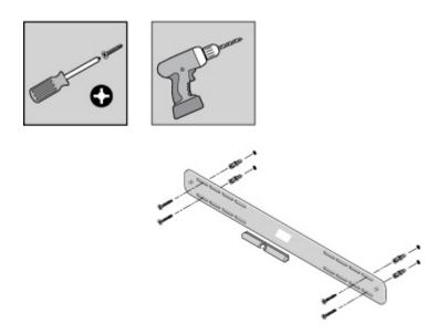
6. Place the bracket on the wall and loosely tighten the screws to secure the bracket. Check with a level and then tighten the screws.
