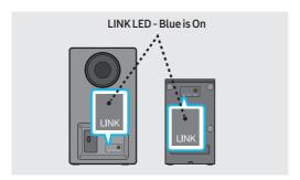
When the connection is successfully established, the blue indicators on the rear of the subwoofer and surround speakers turn on without blinking.
